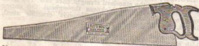
No. 75S REVOLOC —26 in. ship carpenter's hand. Special cast steel, polished blade, skew back, taper ground, carved and varnished beechwood handle, 4 brass screws, 7, 8, 9 and 10 points, is about one inch narrower than regular hand saw, w't per doz. 19 lbs. ....per dozen $30.40
