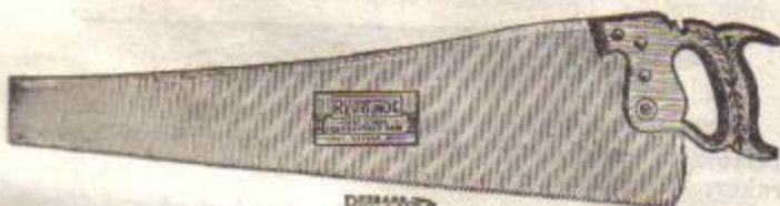
Extra cast steel, grained blade, skew back, mahogany finish, carved handle, polished and etched, 4 brass screws.
